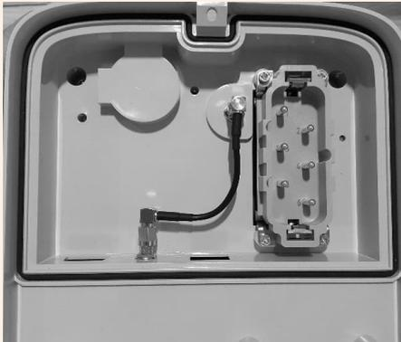
**Anschluss der internen Antenne**
